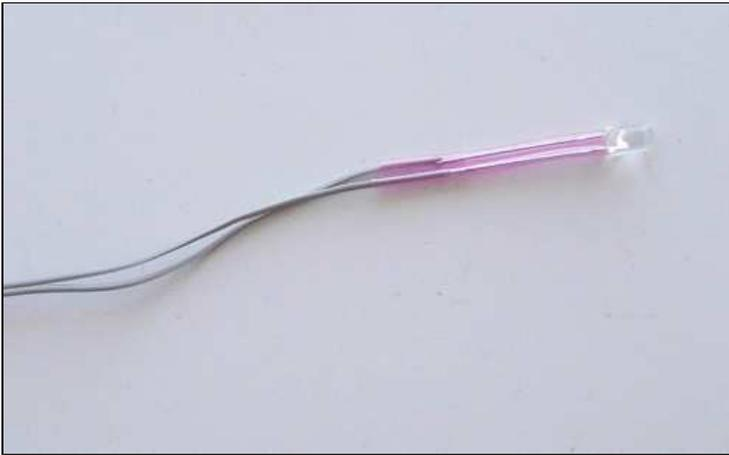
Wrap the LED in bubble foil. Try to fold the foil such that there is a lot of foil in front of the lens of the LED and not so much foil behind the LED. Remember the light needs to be defused by the foil for this to be effective the light has to go through several layers of bubbles and plastic foil.
